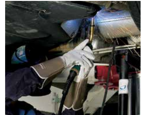
Trim of welding parameters using the Dialog torch
